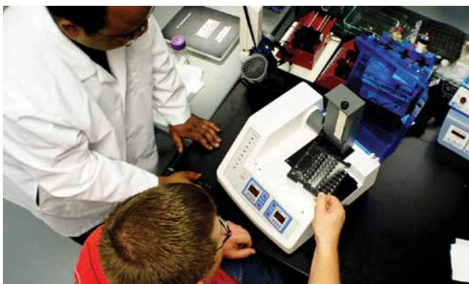
The GPR-800 instrument employs a single-use plastic chip and reagents kit to perform the simultaneous recovery of eight protein samples in 20 minutes
