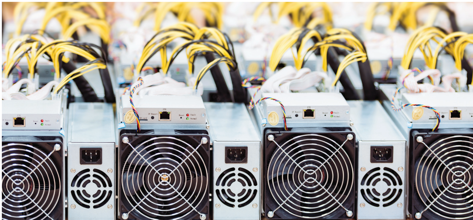
Application-specific integrated circuit (ASIC) rigs used for cryptocurrency mining.
